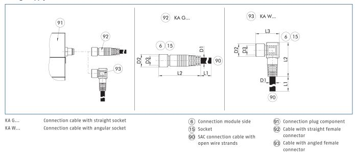
The connection cable is ideal for connecting the corresponding components to the controller or the power supply unit. The connection cable has a 4-pin M8 socket on one side and an open wire strand on the other side for individual connections. The connection cables are suitable for use both in the cable track as well as in torsion applications.
